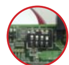
The ID is programmed by a 4-digit DIP switch
