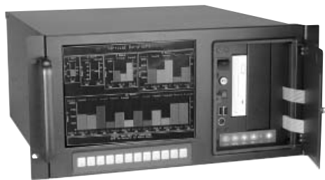
Front view of drive bays and power switch
