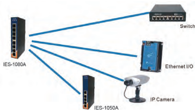
Connections of Ethernet devices
