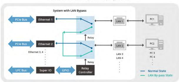
Bypass function enabled allows two LAN ports to be linked together to shunt network traffic, hence important traffic flow where contains critical business data can continue without interruption when one of these LAN ports fails due to power outage or system failure.
