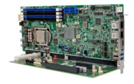
Standard PICMG 1.3 SBCs have several advantages over non-standard SBCs. Firstly, they are more maintainable than a motherboard system and have a much lower mean time to repair (MTTR). Secondly, it is easy to upgrade to a newer or faster processor if desired.
