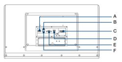
A. RX (RJ-45) B. DP C. 24V<sub>DC</sub>-Power Supply D. 2 x USB 2.0 E. Type B USB (Connect PC) F. HDMI
