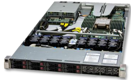
Figure 7 - CloudDC 1U Single Socket Server
