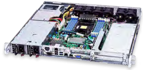
1U UP short-depth server with front I/O
