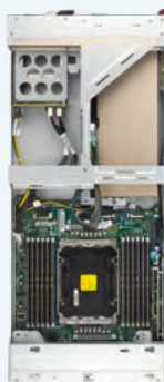
6U SuperBlade 10 UP Nodes in 6U SBI-612BA-1NE34 12 DIMMs, 6 NVMe SSDs, 2 GPUs
