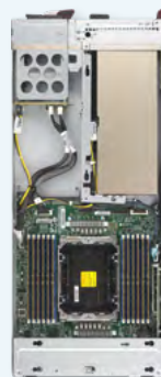
6U SuperBlade 5 UP Nodes in 6U SBI-612BA-5NE34 12 DIMMs, 6 NVMe SSDs, 4 GPUs
