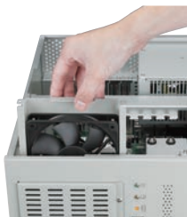
Easy-to-maintain cooling fan
